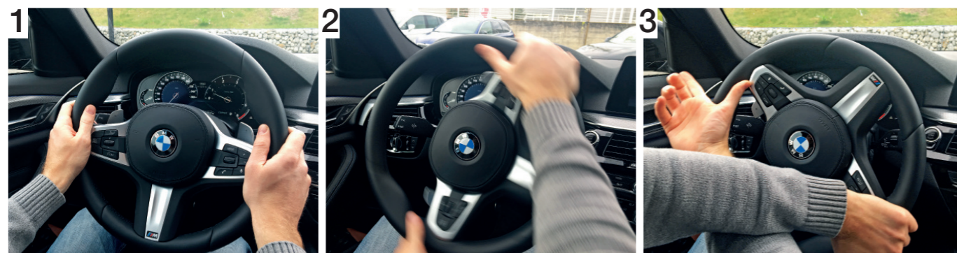
FIXED GRIP STEERING 1. Fixed-grip 'Home' position, with hands set at 'quarter-to-three'. 2. Getting near the limit of fixed grip comfort. 3. The classic pretzel – the absolute limit of the fixed grip technique.
